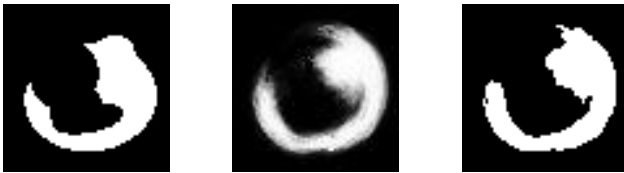
Fig. 6. From left to right: 64 \times 64 original, gray level reconstruction and rounded reconstruction using a full-image network, with absolute total errors 413.7 and 291, respectively
