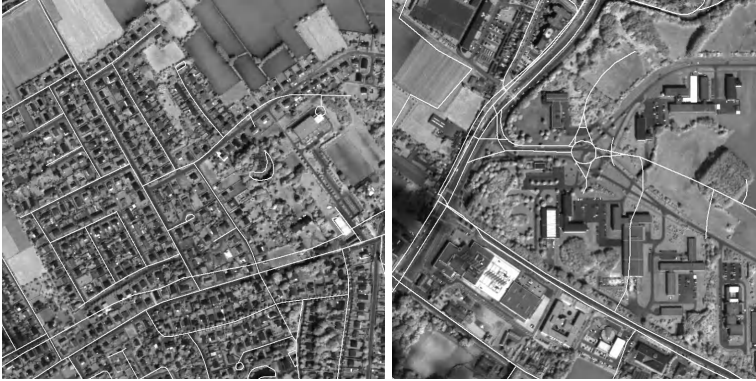
Fig. 1. Example satellite images with the road data in overlay. Local inconsistencies between the two datasets are apparent.
