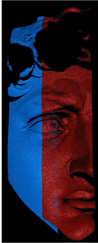
Fig. 11. Points from two scans (“blue” and “red scan”) rendered with lighting
